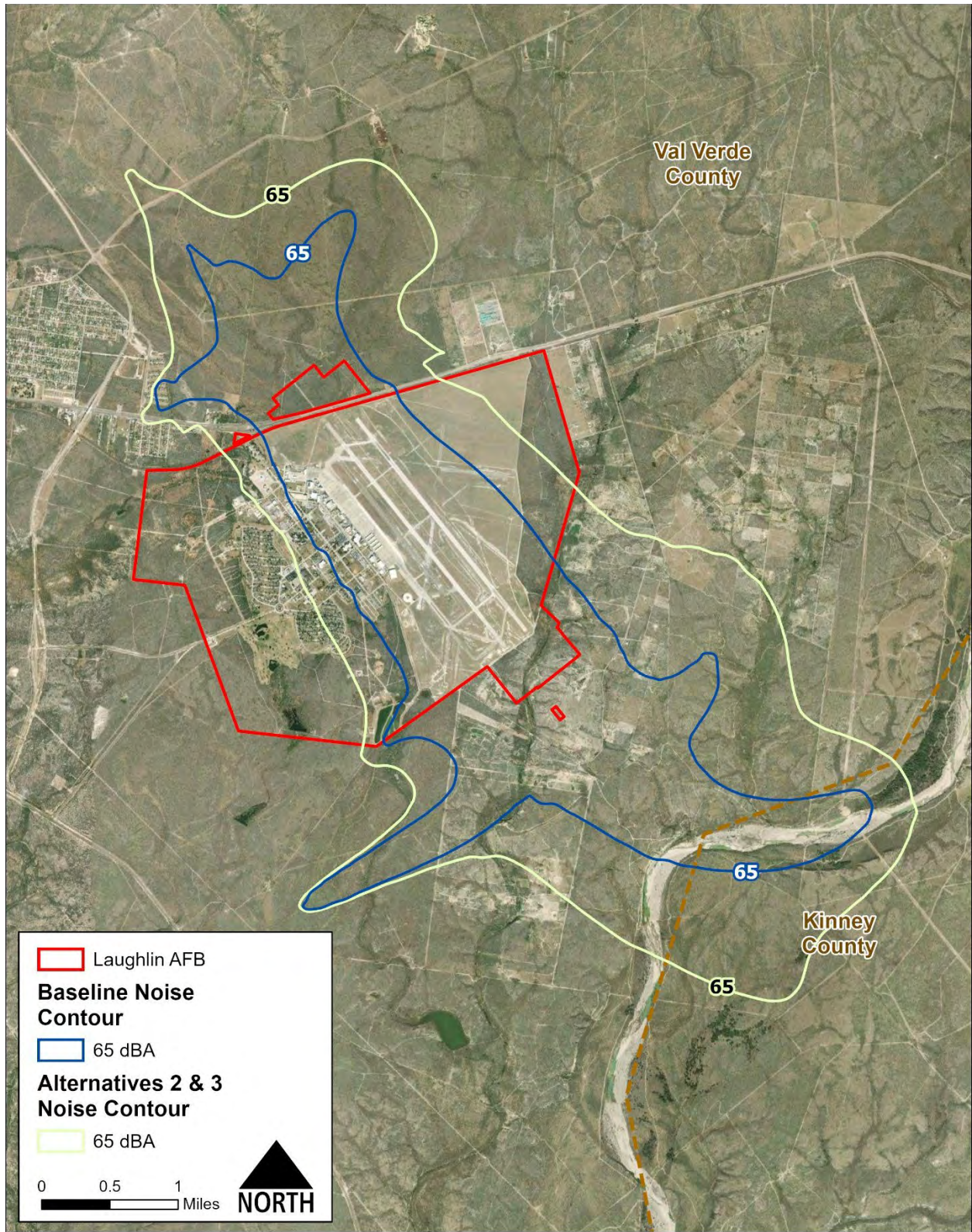
Figure 3-8. Comparison of the 65 dB DNL Contours for Alternatives 2 and 3 and Existing Conditions at Laughlin AFB
